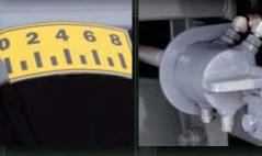
The deck plates are hydraulically controlled from the combine seat for easy adjustment.
